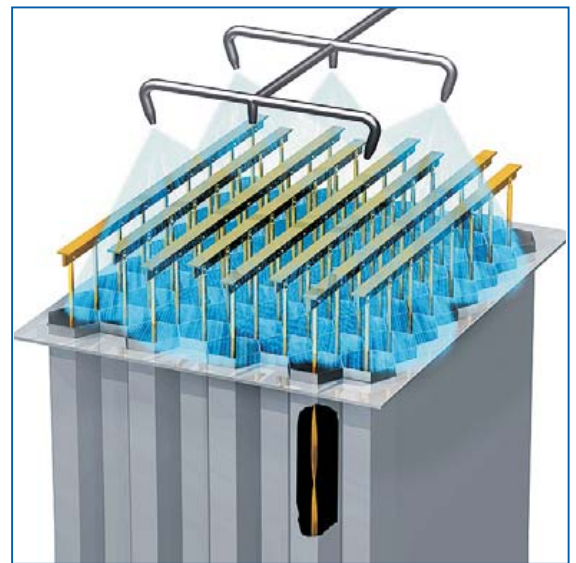
Electrodes cleaned by periodic flushing system
